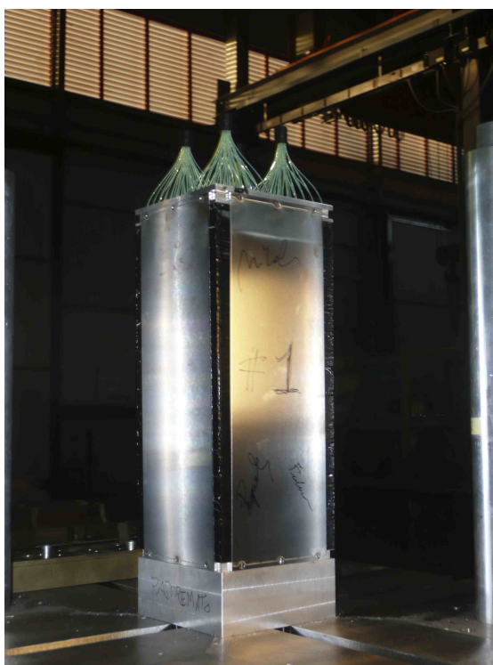
Fig. 4: The first 1.5^\circ tapered module of the EMCal generation II prototype produced in EU shown. The module's internal compression is maintained by a set of 5 Bellville washers (non linear springs) acting between the top and bottom containment Al plates to prevent the delamination of the internal Pb-scintillator sandwich.
