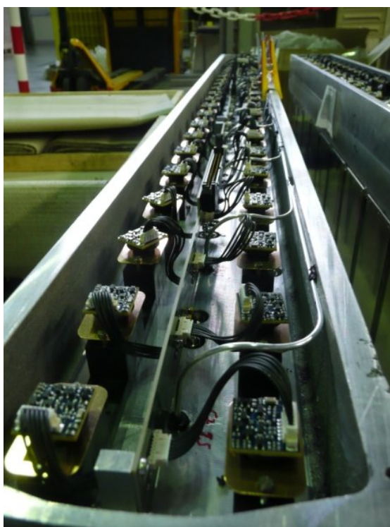
Fig. 3: View of a fully assembled strip module. The photo shows the APD+CSP package and copper shielding mounted light guide fixture. On the right part of the photo the LED UV optical fiber distribution system is visible. Each strip module, is cabled via 3 T-Cards visible in the center of the assembly.
