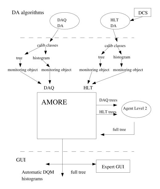
Figure 3: AMORE calibration flow for the TPC
